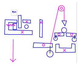
the run button) is pulled up, the spring forces the ball to the right, it falls onto the see-saw, allowing the wedge to drop, cracking the egg into the frying pan. But if we simply run the simulation, nothing interesting happens: the stopper, responding to gravity, simply drops down a little, as does the ball, which then stays put. We need to be able to tell the system what is supposed to happen.
