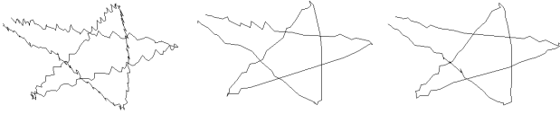
Figure 1. A very noisy stroke along with the fits generated using curvature and speed data with average based filtering. Both fits have picked many false positives due to noise.
