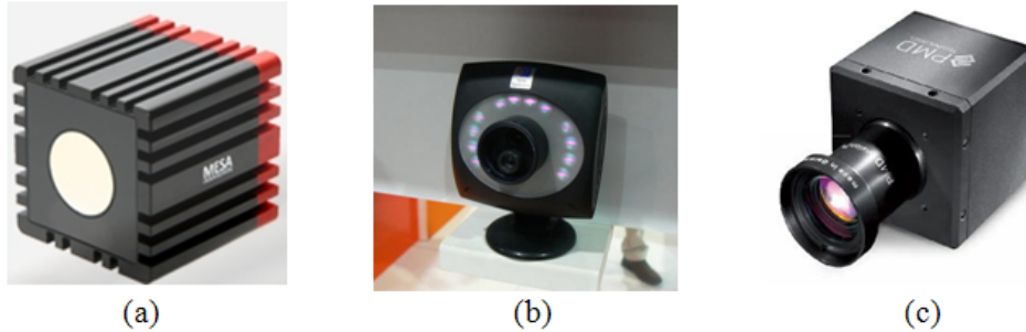
Figure 3-1: Various kinds of time-of-flight cameras. (a) SwissRanger SR-4000, (b) 3DV ZCam, (c) PMD Vision CamCube 3.0
