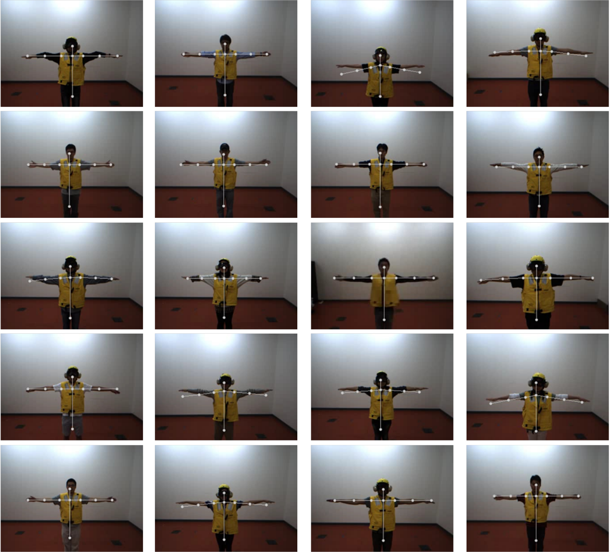
Figure 4-11: Initialization results collected from 20 subjects. Although each subject has made a T-pose for the initialization, the shoulder angles were not always 90 degree to the backbone, preventing us to assume that the chest point is always at the middle of two wrist points.
