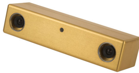
Figure 3-2: Bumblebee2 stereo vision camera from Point Grey Research Inc.
