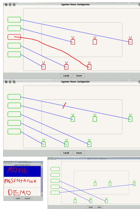
Figure 2. Usage examples. Top: making a new connection. Middle: removing a connection. Bottom: loading a saved configuration.
